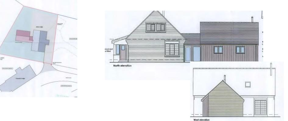
•Full planning permission is sought for an extension to the rear of an existing timber , rectangular shaped house within Ballater.
